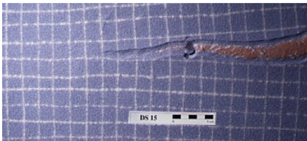
Fig. 1. Sandbox experiment of normal extension shows the propagation of a rift in the brittle layer (gray) without interruptions. An elongated diapir ascended from the ductile layer into the rift. Scale bar in cm.
